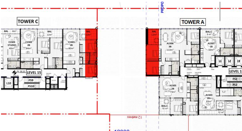
Figure 22 - Recommended building separation at Levels 9 and above between Tower A and Tower C. Source: Adapted from Plan A0104 (Rev F) as prepared by Koichi Takada Architects.
