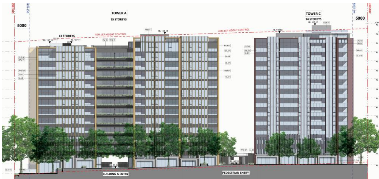
Figure 25 – North-west elevation showing height non-compliances at Towers A and C from Herring Road. Source: Plan A0200 (Rev G) as prepared by Koichi Takada Architects.
